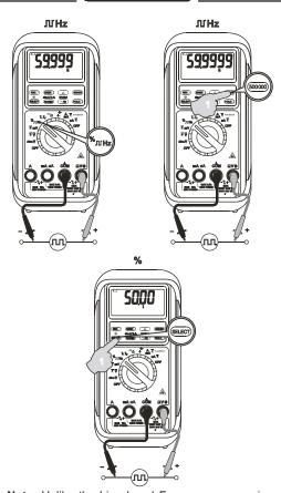
**Note:** Unlike the Line Level Frequency measuring function as previously stated, this Logic Level Frequency function is set only at the highest input sensitivity to measure digital type electronic signals.
