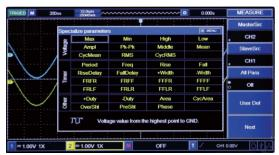
Automatic Measurement of Waveform Parameters
